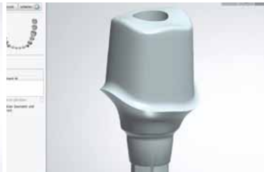
Abb. 23: Das virtuell designte Abutment.
